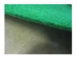
Short Fibre, Thickness 3-5 mm, EV3 reflected light reading 3 or above
