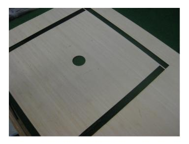
A template can be made from a single veneer of wood(shown) or thin ply wood. It can either be laser cut or cut using a sharp knife
